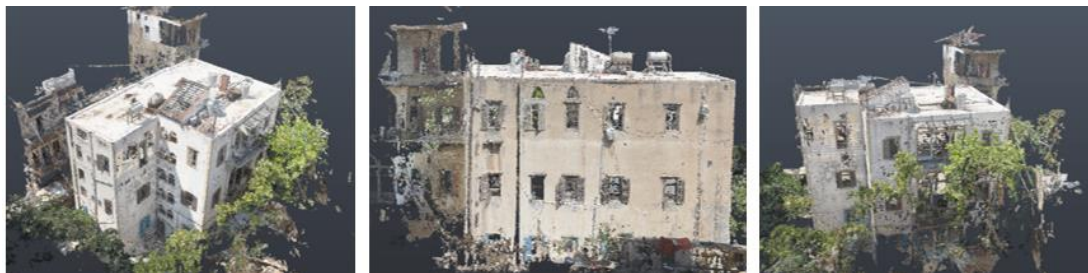
Fig 15. 3D of the pointcloud model for the (695) block Rmeil Source: photos from DGA, developed by the author.
