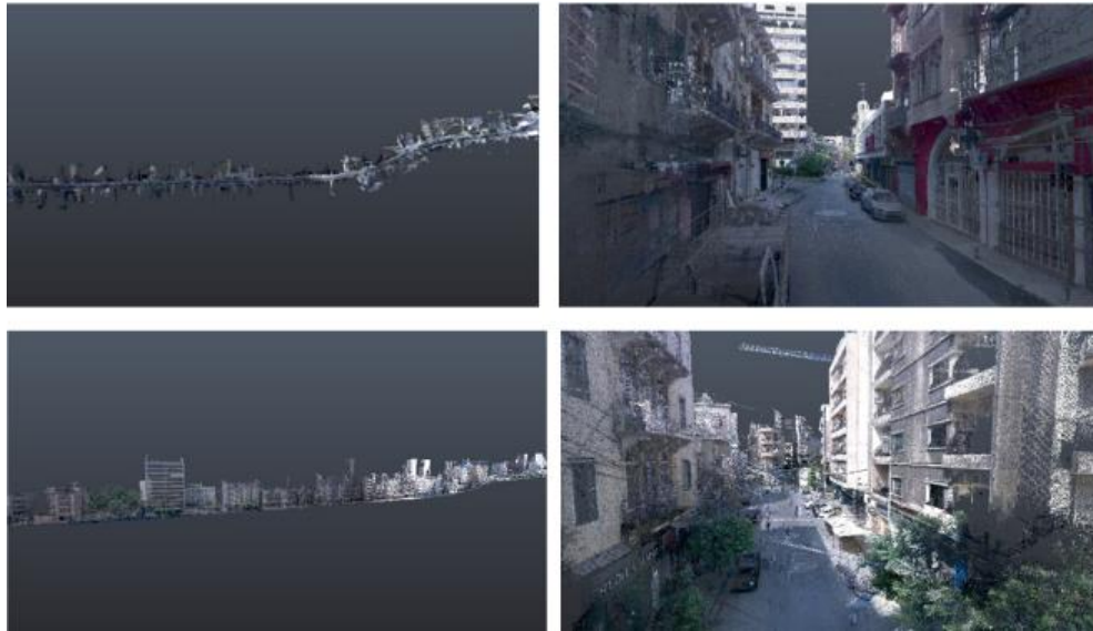
Fig.6: Point cloud top view & perspective (UAV- TLS) Armenia Street after the POB's 2020 Source: (X,Y,Z) Lebanon.
