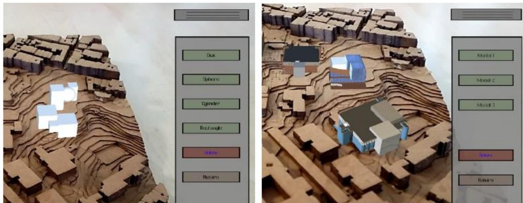
Fig.3: 3D modelling by using basic geometric forms on AR environment, on the right. Pre-installed digital models on the physical model, on the left.
