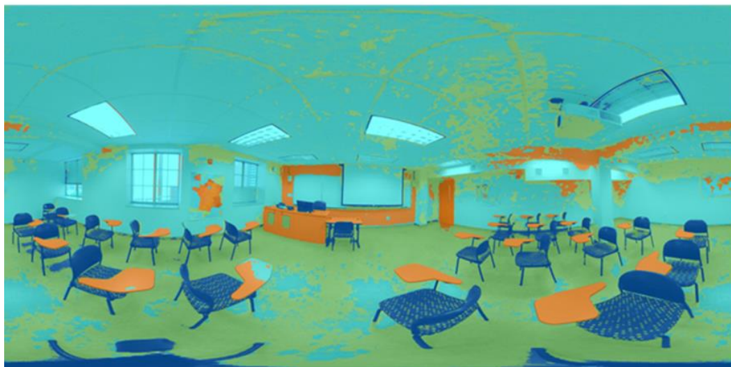
Fig.3: Image segmentation with k-means clustering algorithm using k=4 segments. Each segment refers to different semantic elements in the scene.
