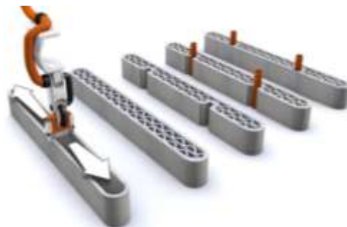
Fig.13: Schema of built walls by CC and placing the passages for the needed installations.
