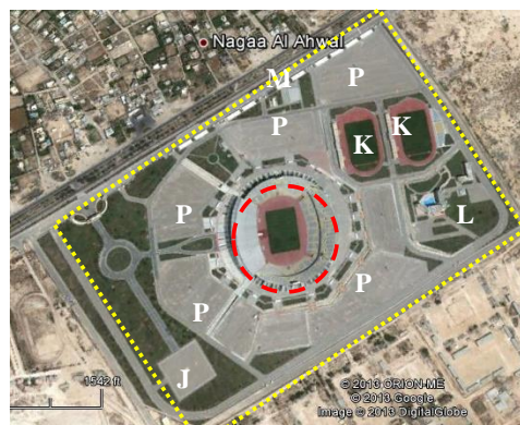
Fig 41 46 : Yellow line: 3.5m high fence has 10gates. Red line: 1.2m high fence has 17gates.
