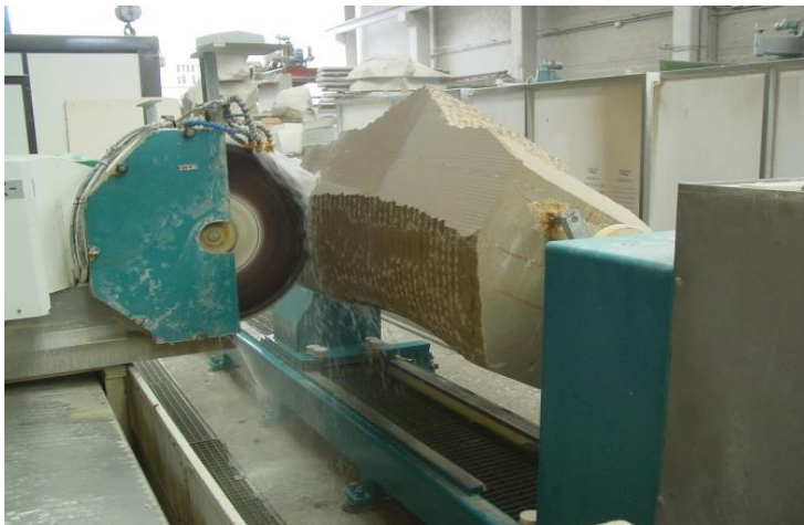
Fig.2 Horizontal pivot numerically controlled and machine specially adapted for the fabrication of a stone component of multiple ruled surfaces for the Basilica of the Sagrada Família
