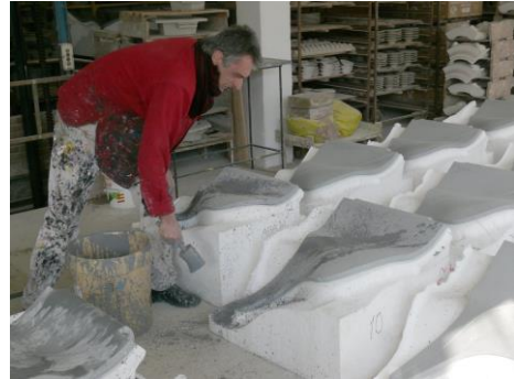
Fig. 6 The shaping of the ceramic tile Reference: Cloud 9 Architects
