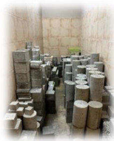
Fig.4: Curing the concrete samples.
