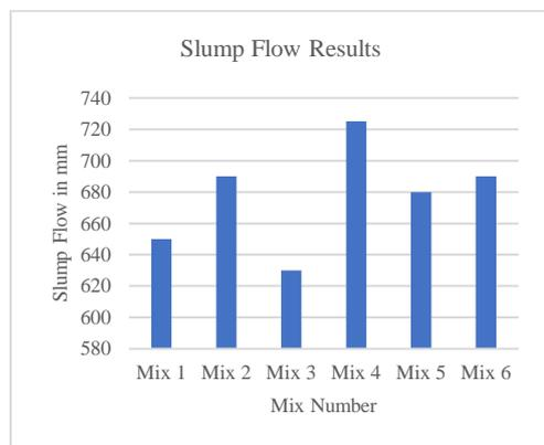
Fig.10: Slump Flow Results
