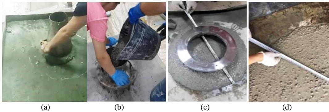
Fig.8: Slump Flow, Visual Stability Index (VSI), J-Ring, and  $T_{500}$  Tests
