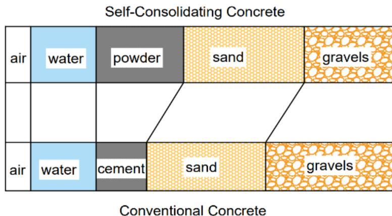
Fig.1: Components of Self-Consolidating Concrete Compared to Conventional Concrete
