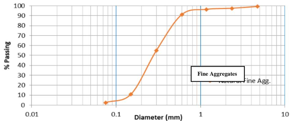
Fig.5: Sieve Analysis for the Fine Aggregates
