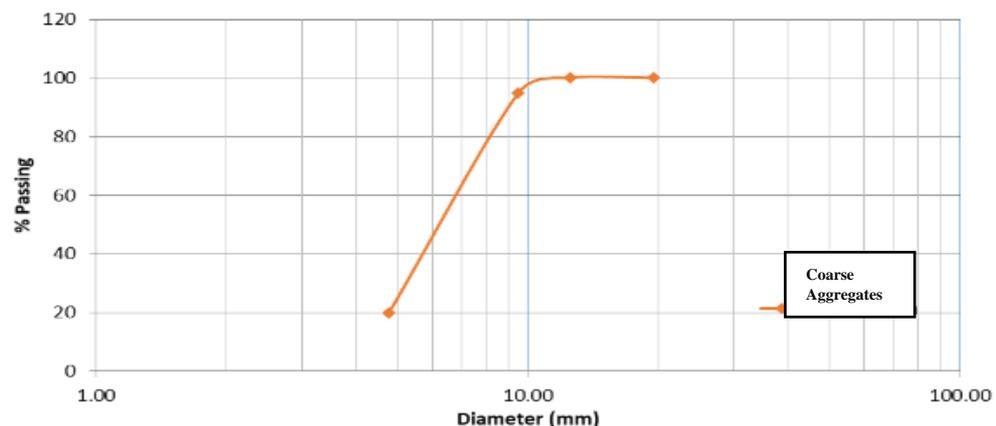
Fig.4: Sieve Analysis for the Coarse Aggregates
