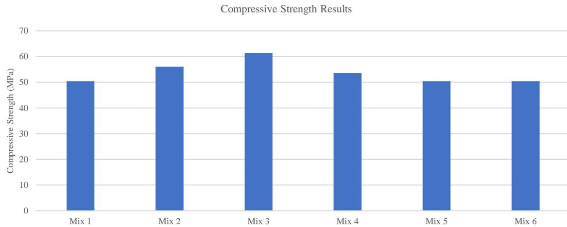
Fig.12: Compressive Strength Results
