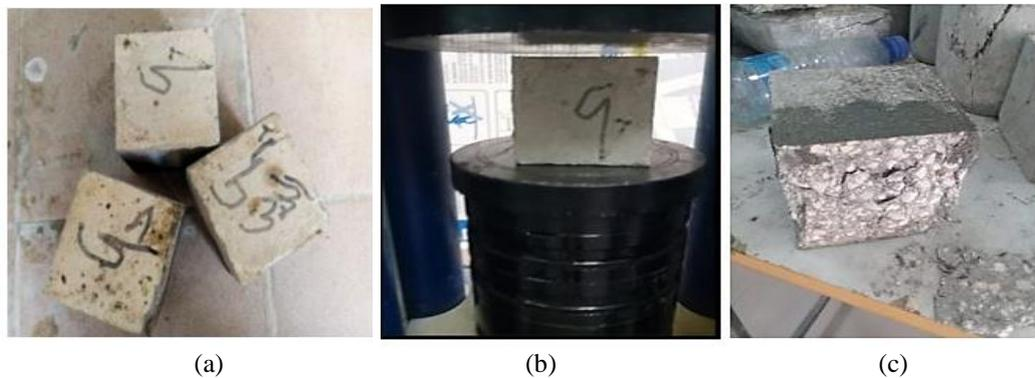
Fig.9: Compressive Strength Test
