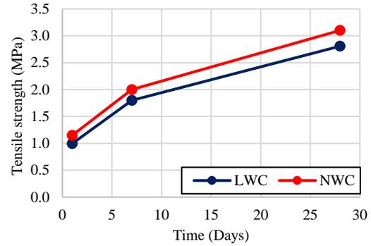
Fig.10: tensile strength for LWC and NWC.
