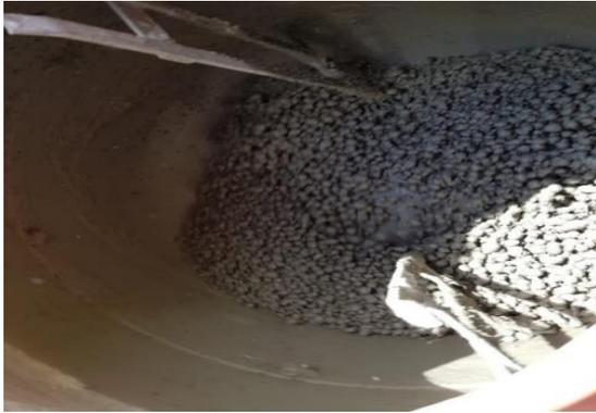
Fig.1: Lightweight aggregate under Manufacturing.
