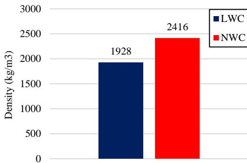
Fig.7: Density of LWC and NWC specimens
