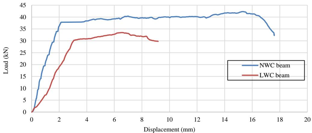
Fig.12: Load – displacement curves for NWC and LWC beams.
