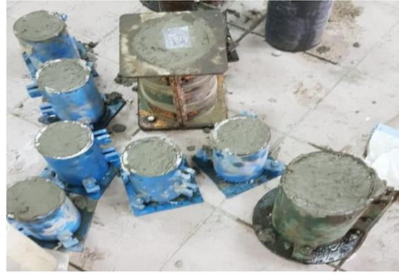
Fig.4: Cylindrical specimens after casting.
