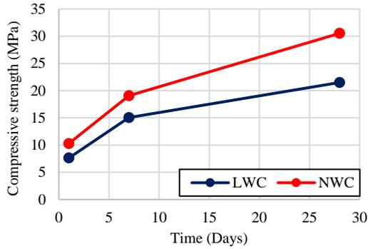
Fig.9: Compressive strength for LWC and NWC.
