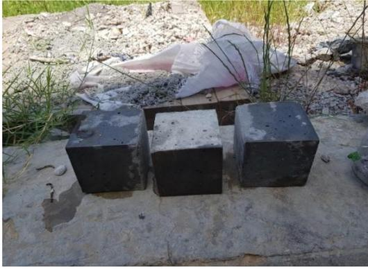
Fig.3: Concrete cubes after curing.
