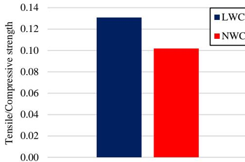
Fig.11: Tensile/Compressive strength ratio for LWC and NWC.
