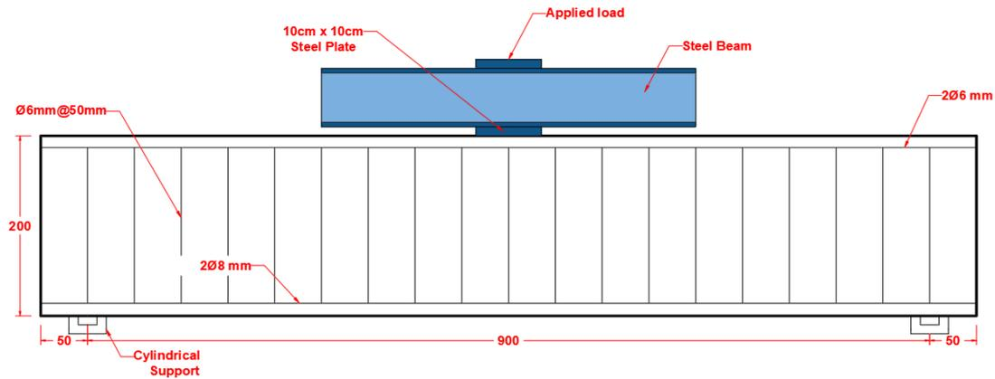
Fig.6: Three – point bending test details.
