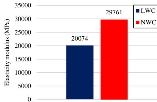
Fig.8: Elasticity modulus for LWC and NWC specimens.
