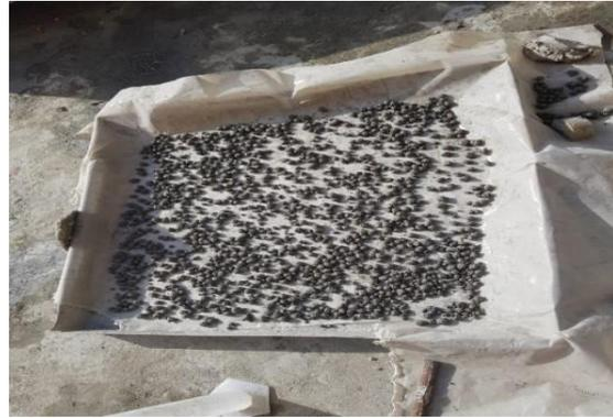
Fig.2: Fresh sample of lightweight aggregates.
