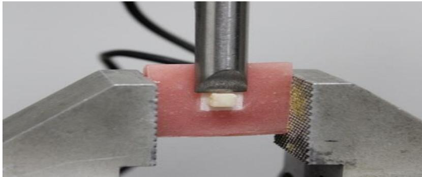
Fig.1: Chisel of Universal Testing machine applied composite/zirconia interface during testing of SBS.
