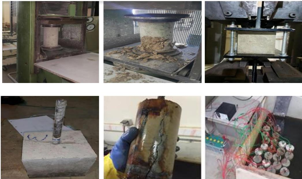
Fig.2: Compressive strength, pull out, and accelerated corrosion tests
