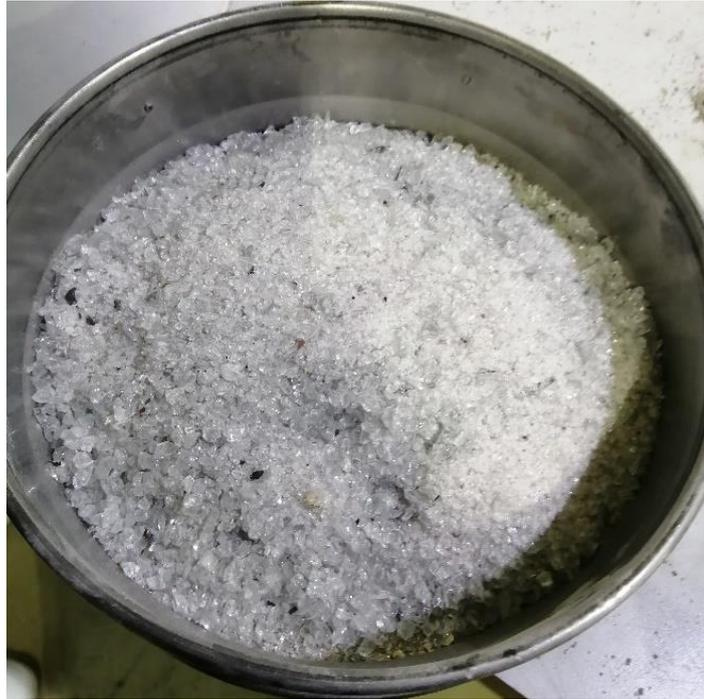
Fig.1: Crushed CRT glass
