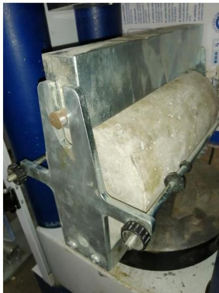
Fig.5: The setup of tensile splitting strength testing
