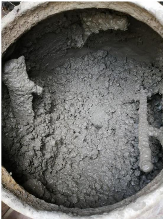
Fig.3: Concrete after mixing in the pan mixer
