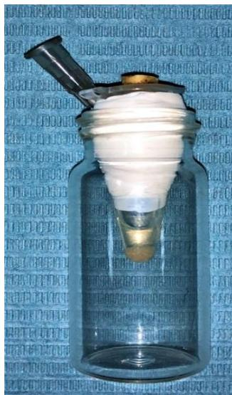
Fig.1: Shows the apparatus prepared for the collection of apically extruded debris as described by Myers and Montgomery (1991).
