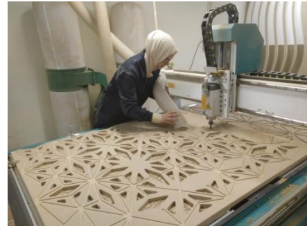
Figure 1: Digital fabrication of panels Source: by authors.
