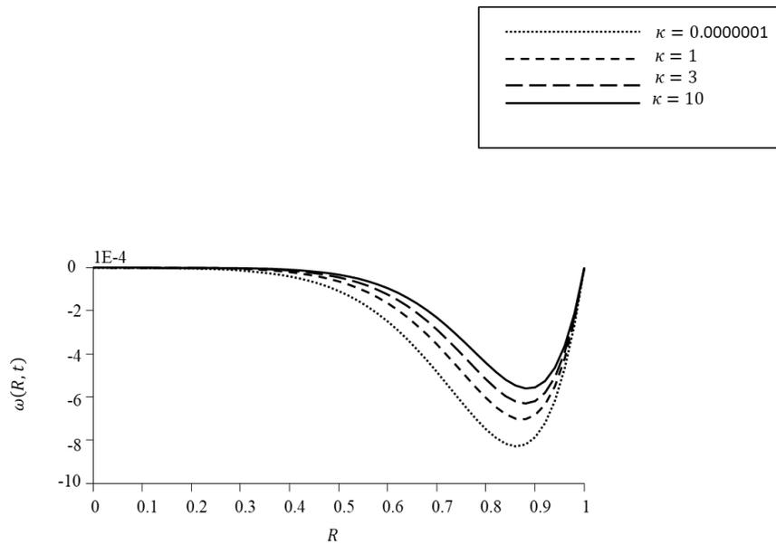
Fig.4: Variation of microrotation  $\omega(R, t)$  versus distance for  $t = 0.03$  for case 1.
