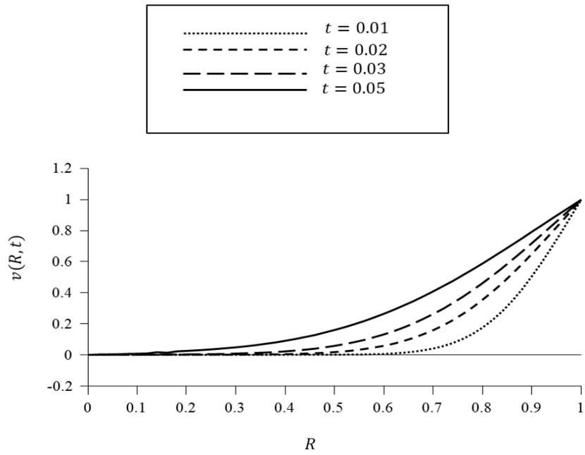
Fig.11: Variation of velocity  $v(R, t)$  versus distance for  $\kappa = 1$  for case 3.
