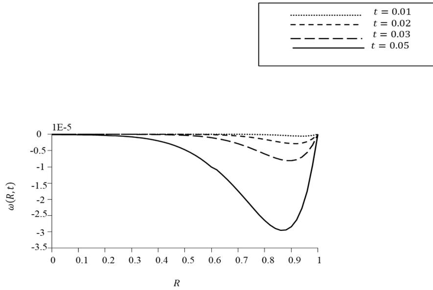
Fig.7: Variation of microrotation  $\omega(R, t)$  versus distance for  $\kappa = 1$  for case 2
