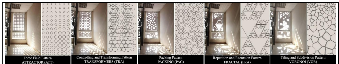
Fig. 2 Structure of all basic parametric patterns integrated with the envelope of the of the office space.
