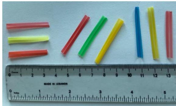
Fig.1: Shredded waste plastic straws (WPS).
