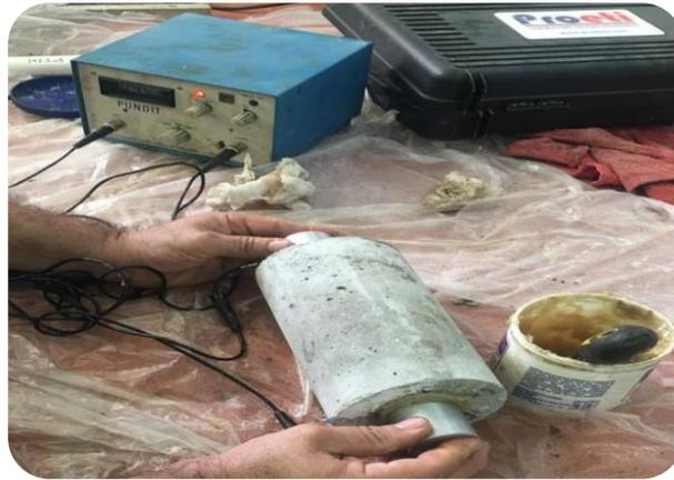
Fig.7: Pulse velocity of the concrete specimens.
