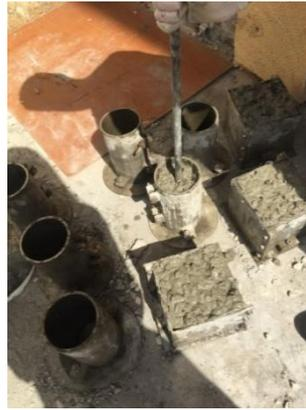
Fig.3: Compacting using a tamping rod.
