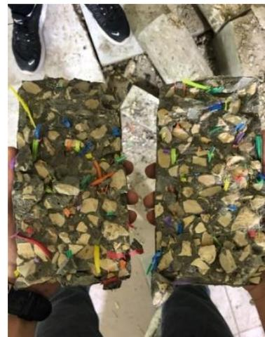
Fig.12: Fiber distribution after testing for PS-0.5 sample
