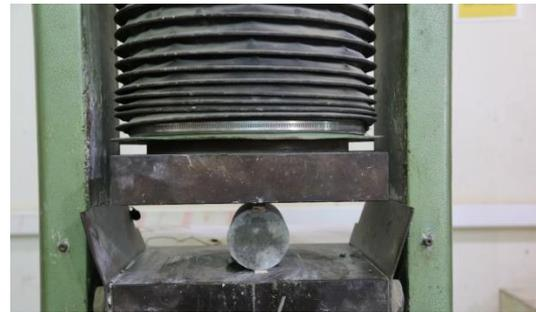
Fig.6: Specimen under splitting tensile test
