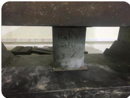
Fig.5: Specimen under compressive strength test
