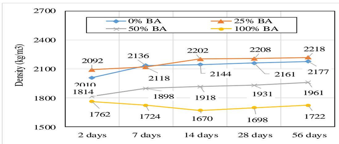
Fig.5: Effect of MSWIBA on mortar density
