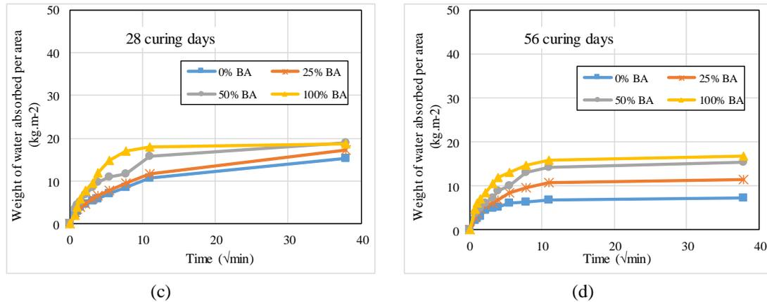
Fig.8: The effect of MSWI-BA on the capillary water absorption with time (sqrt) at different curing durations. (a) 2 days (b) 7 days, (c) 28 days and (d) 56 days
