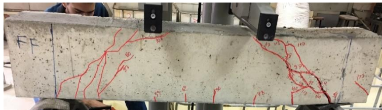
Fig.12: Beam (B4) at failure
